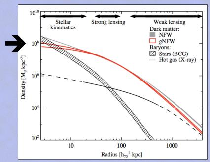
Weak lensing mass maps (Subaru) combine with strong lensing constraints (HST) and resolved stellar velocity dispersions of the cluster cD (Keck) to infer the DM density profile over 3 decades in radius (3 kpc - 3 Mpc)
