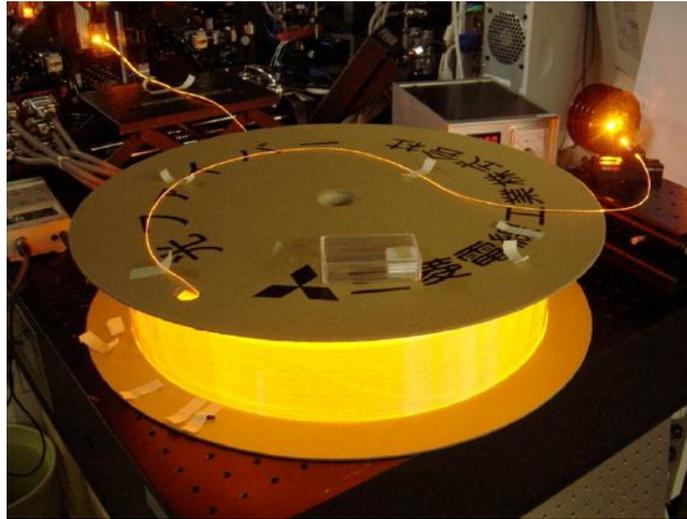
**Figure 3.** The experiment of laser input into the prototype PCF.
