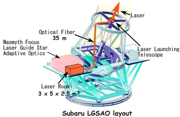
**Figure 1.** The layout of Subaru laser guide star adaptive optics with 188 elements.
