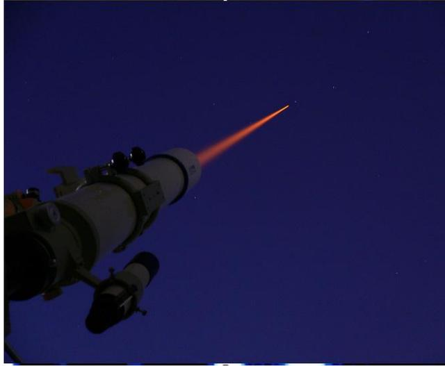
**Figure 7.** Laser projection experiment in Japan. Projected output power in the air is about 0.5W. The beam size is about 10 cm
