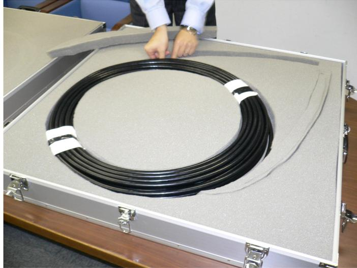
**Figure 2.** The photograph of PCF cable in real use on the Subaru Telescope.
